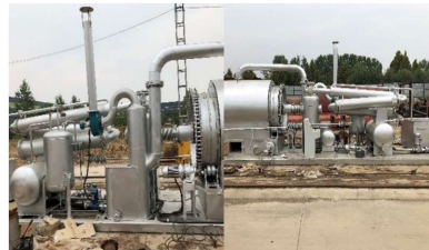
Rotating Drum Reactor
