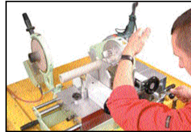
Peeling the pipe
