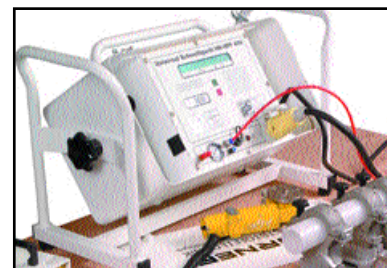
The completed joint cools in the clamps
