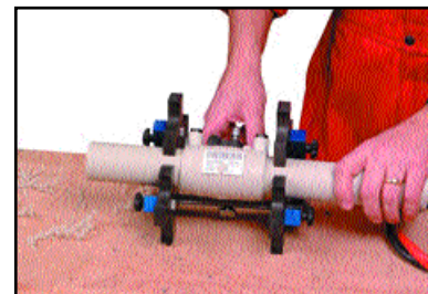
Once cooled, the joint can be removed
