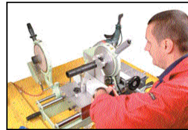
Peeling the pipe
