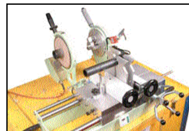
Cooling the completed joint before handling
