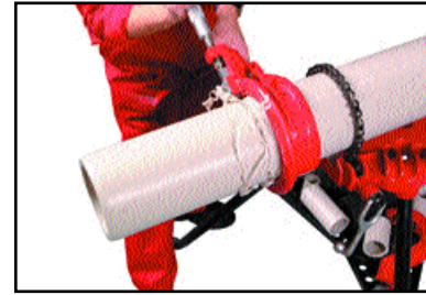
Cutting the pipe with a rotary pipe cutter
