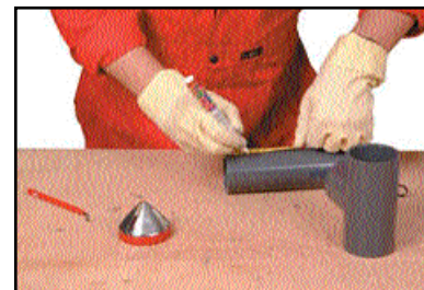
Marking the pipe end
